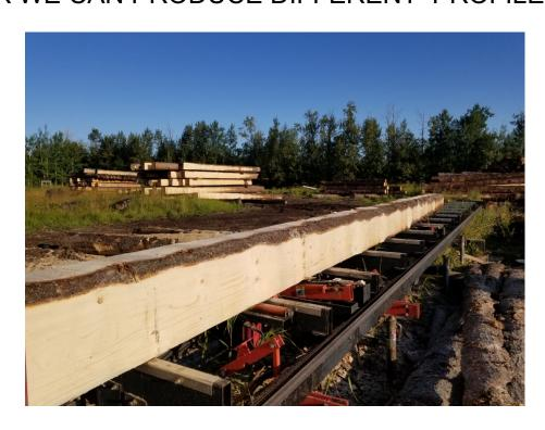
WE CAN SAW TIMBERS UP TO 40 FEET ON OUR FULLY HYDRAULIC TIMBERKING BANDSAW (GREAT SAW AND COMPANY)
